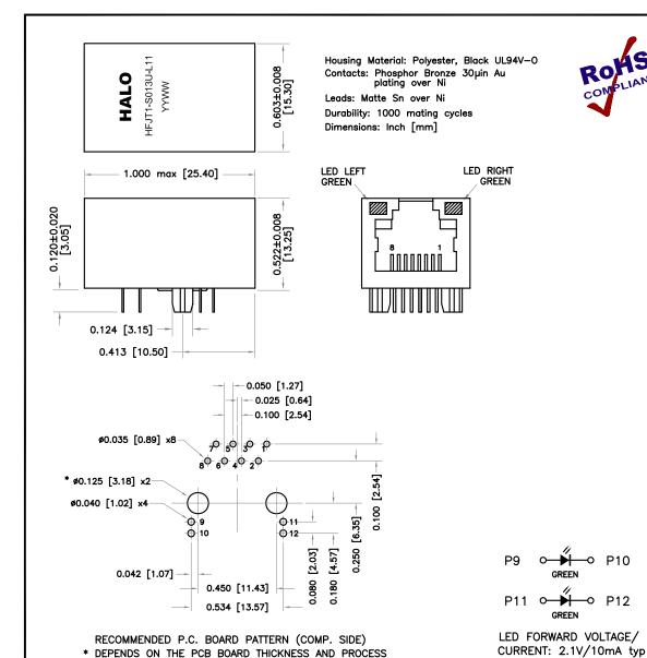
TOLERANCES, ADJUST THE NOMINAL SIZE TO ENSURE A SNUG FIT
